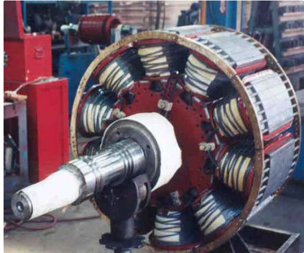
Figure 1: Salient Pole Synchronous Rotor
