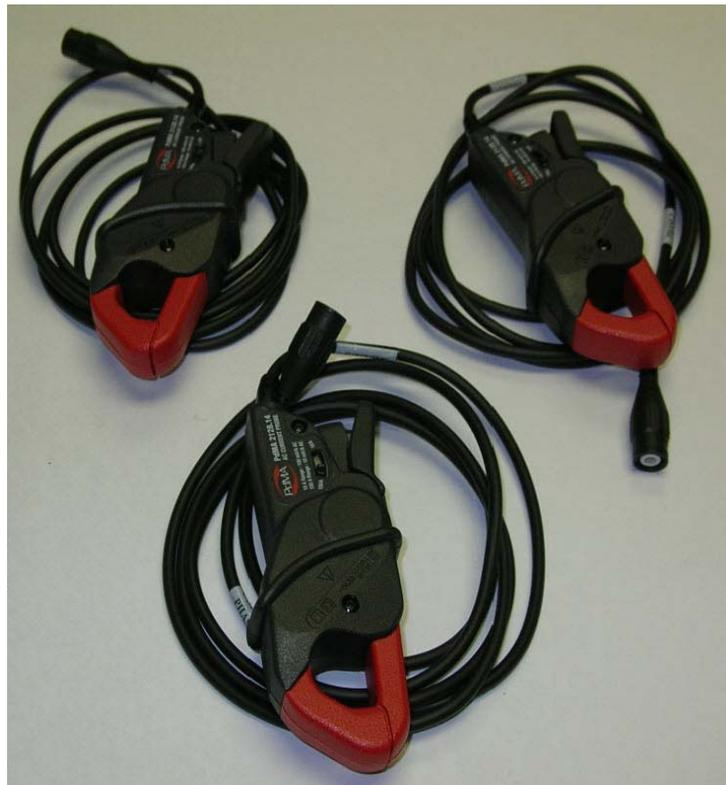
**Figure 2-10: EMAX Current Test Leads**
