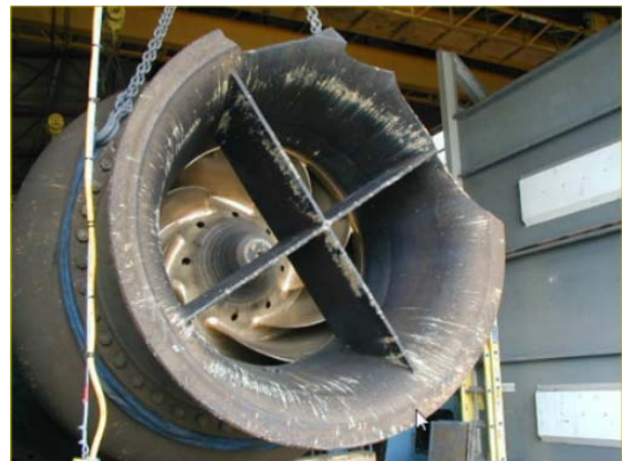
Figure 8. Damaged inlet bell on circ water pump.
