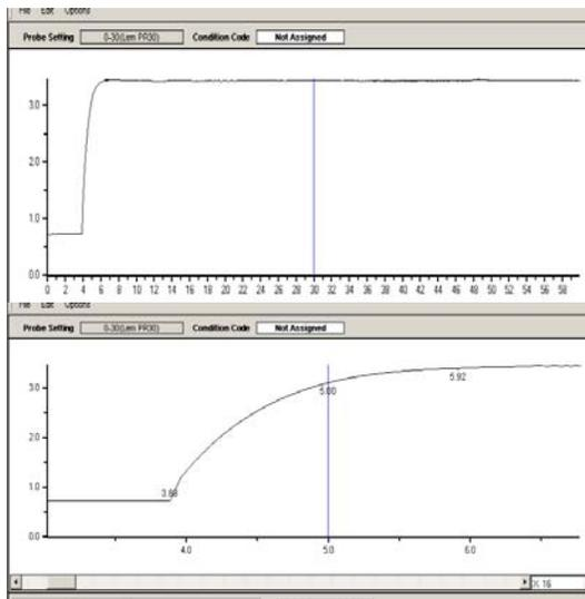
Figure 2: Amps vs. Seconds - Energizing the Field Circuit
