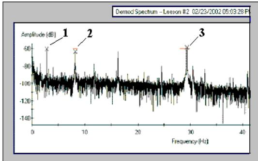
Increasing Fp indicates possible rotor degradation, such as cracked or broken rotor bars or end rings. Fp is also used for speed acquisition. (See point 1)
