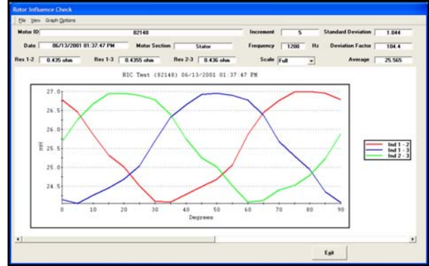
Figure 13. Repeated Variations Throughout All Three Phases of Inductance
