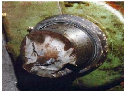
Figure 2- Rod mill pinion shaft failure.
